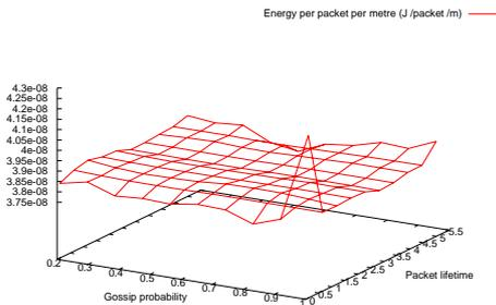
Figure 4: Observed energy per packet per metre vs gossip prob. and packet lifetime
