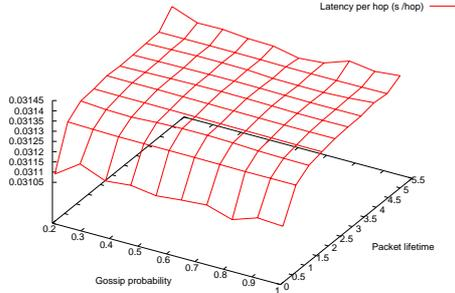
Figure 3: Observed latency per hop vs gossip prob. and packet lifetime
